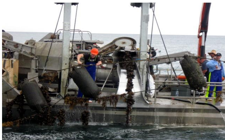
Figure 9: Showing harvesting process of rope grown mussels
